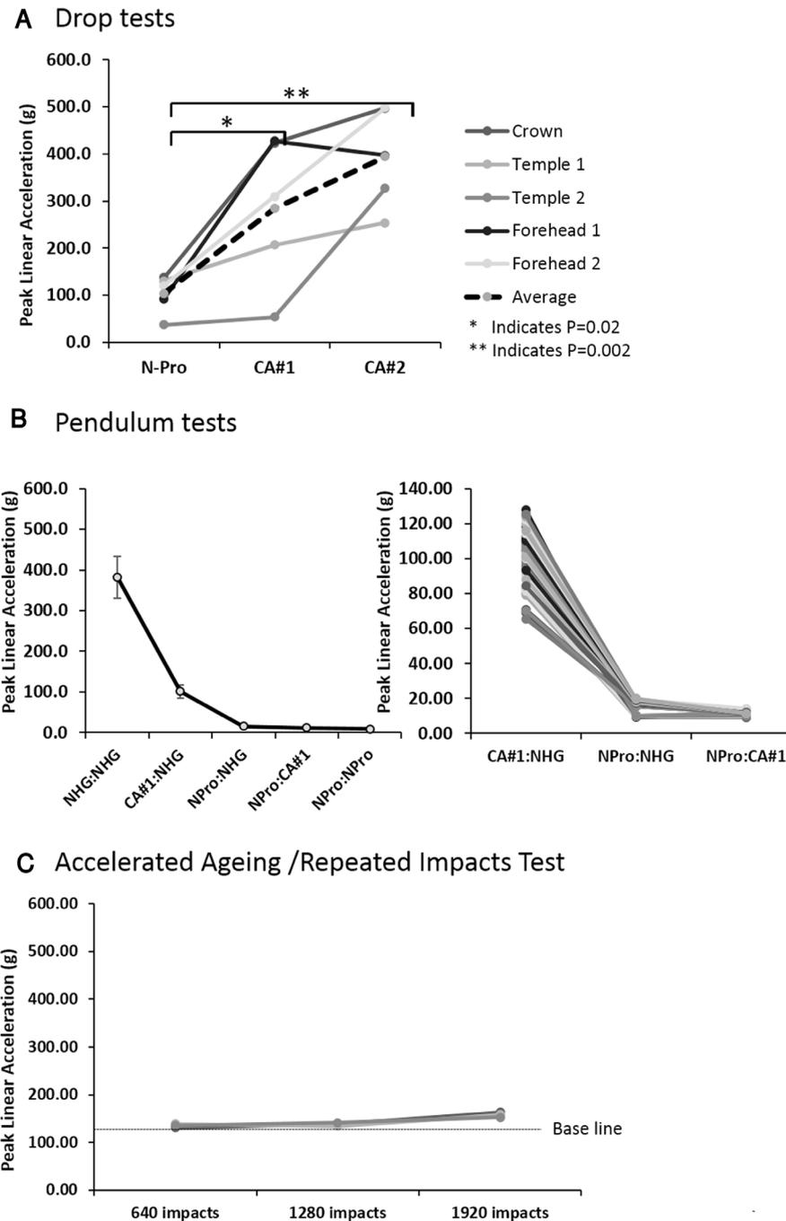
**Figure 3** (A) Average measured max *g* force following drop tests on forehead, temple and crown sites of head-forms with N-Pro, CA#1 and CA#2. (CA#1 and CA#2=commercially available head guard 1 and commercially-available head guard 2, respectively). (B) Average measured max *g* force in pendulum tests with two headforms. (C) average measured max *g* force prior to testing and after 640, 1280 and 1920 impacts to the N-Pro head guard, respectively. NHG, no head guard.
